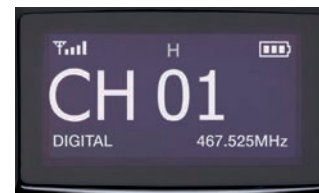
Informative display shows both the channel number and the frequency
